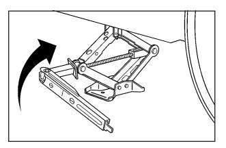
7. Raise the vehicle by turning the wheel wrench clockwise. Raise the vehicle far enough off the ground so there is enough room for the compact spare tire to fit underneath the wheel well.
